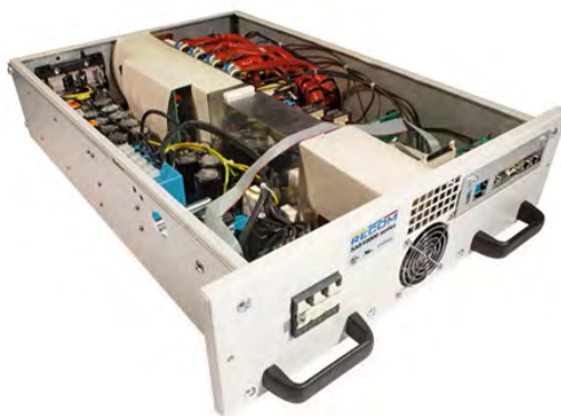
Figure 2: The SAB10000 series provides 10kW of battery charging and is bidirectional
