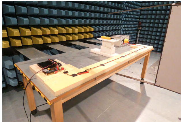
Figure 3: Conducted Emissions test setup
