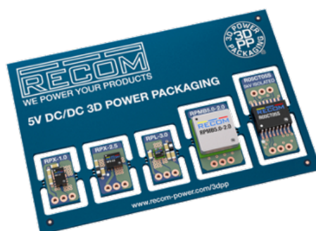
Figure 2: Examples of DC/DC Solutions Taking Advantage of SOTA 3D Power Packaging [13]
